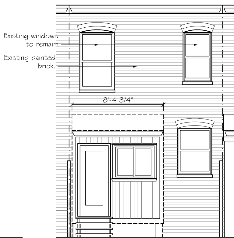
2 Existing Southeast Elevation A-4 3/16" = 1'-0"
